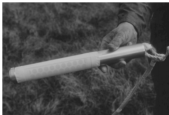
Fig. 1. A gas diffusion sampler. Holes through which gases diffuse are visible beneath the diffusion membrane and a layer of nylon mesh. See text for further details.
