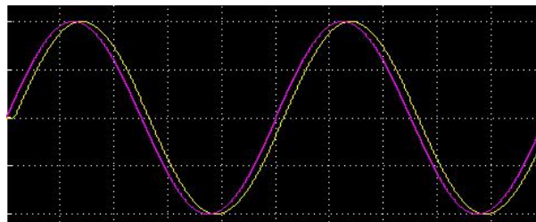
Figure 3 Buffered latency measurement using a mixed signal oscilloscope
